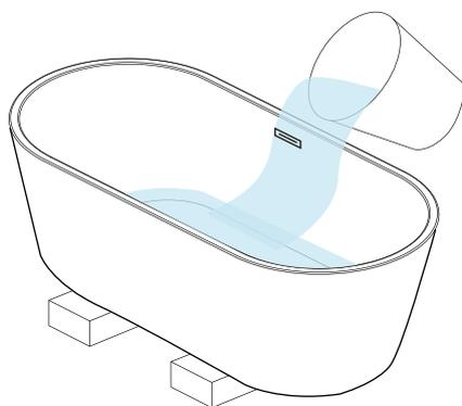
Set your bathtub on two 4x4 pieces of lumber so you can have access from the bottom of the bathtub. Put a tray beneath the bathtub.
