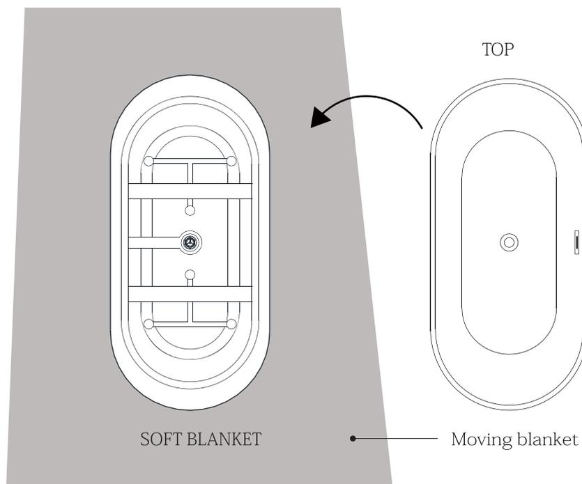
**Step 2** Turn bathtub upside down and set it on a non-abrasive mat, blanket, or cardboard to prevent any scratches on tub rim.
