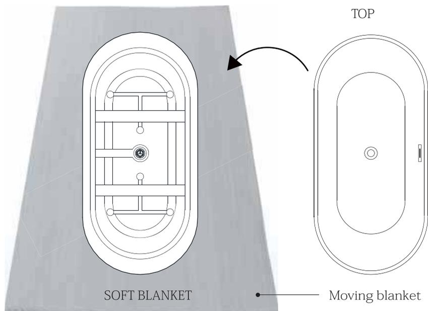
**Step 2** Turn bathtub upside down and set it on a non-abrasive mat, blanket, or cardboard to prevent any scratches on tub rim.
