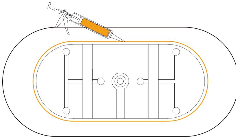
**Step 7** Apply a generous bead of adhesive or waterproof silicone to the bottom of the tub and caulk around the edge of the tub.
