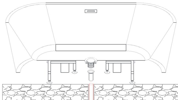
**Step 8** Flip the tub over and carefully set the tub into position with tail piece assembly to waste vent and connect to the drain.
