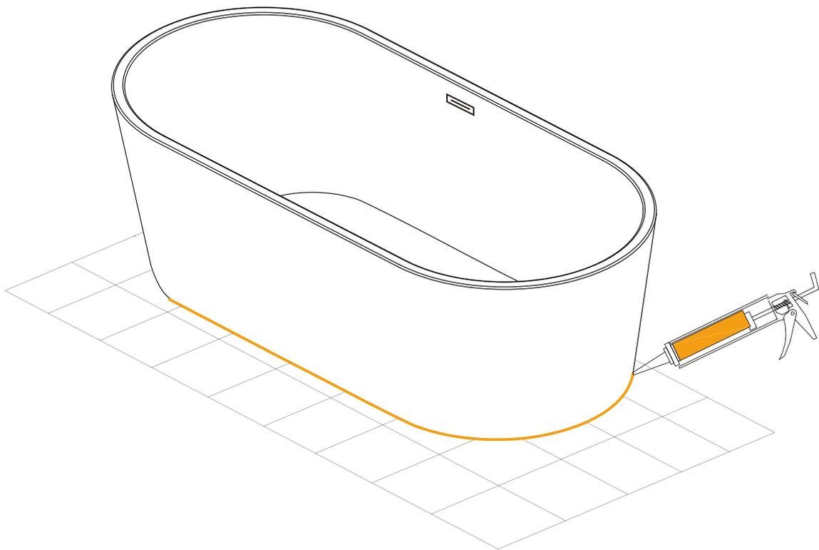
**Step 9** With the tub now set in place, wipe off any excess tub or tile caulking, adhesive where the tub meets the floor with wet cloth.
